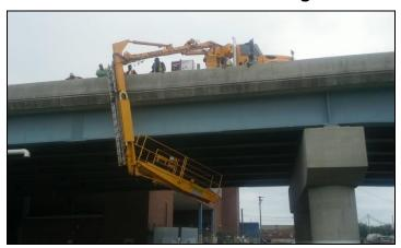
DGS held training for DOT to use their new Paxton-Mitchell SNOOPER® truck which is a bridge inspection and maintenance crane.
